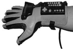
Fig. 5. An instrumented glove (Nintendo power glove)
