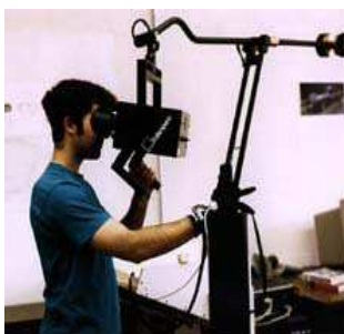
Fig. 2. A Binocular Omni-Orientation Monitor (BOOM)
